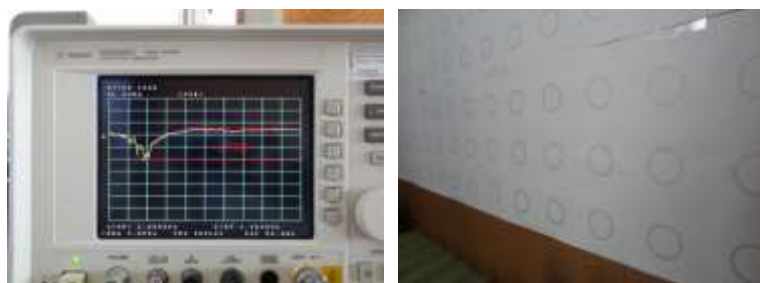
Figure 9: Meta-paper (ring) frequency response; minimum @ 3,0 GHz (left) and meta-paper (ring) (right)
