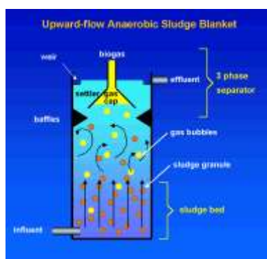
Fig. 6: Principle of the UASB
