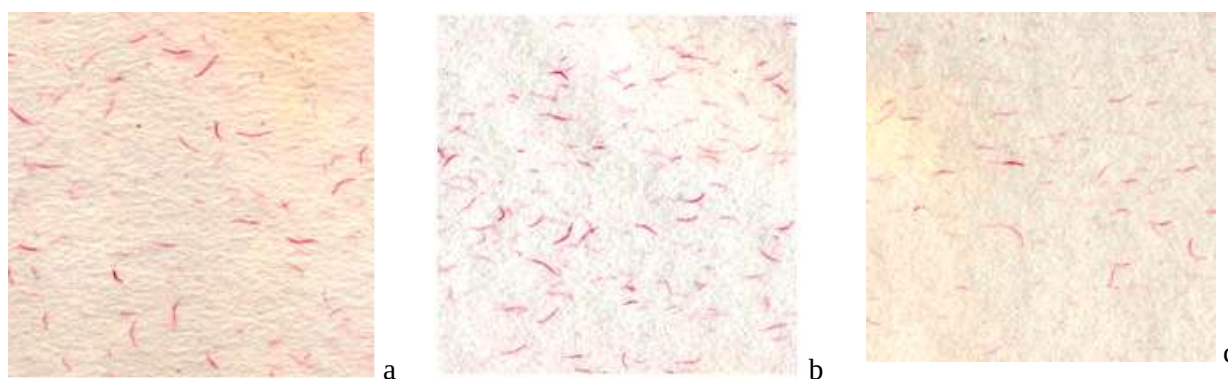
Fig. 1. Scanned images of the anisotropic paper samples of softwood pulp with partially dyed fibers obtained by modes: a – «min»; b – «med»; c – «max»
